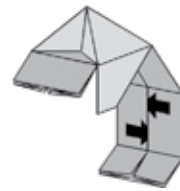
32 Attach two B modules to each A module, making sure that the arms of the B modules go underneath all the layers at the centre of the A modules.
